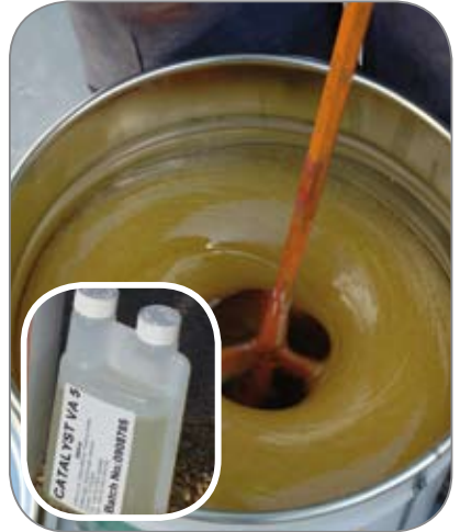
Mixing the base component with a paddle
