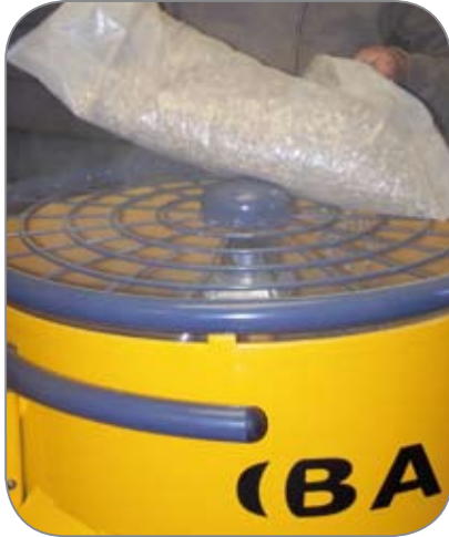
Charge the mixer with aggregate
