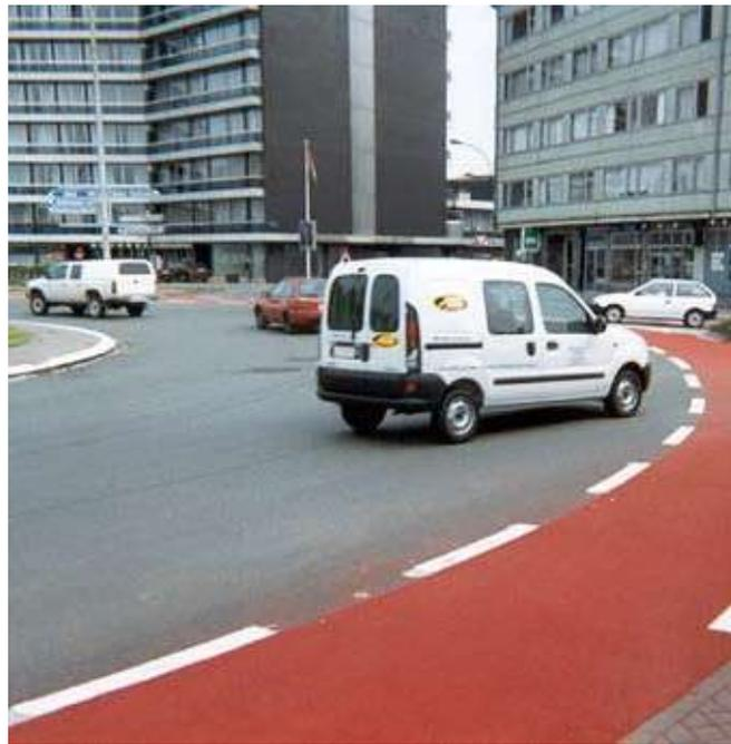
Base aggregates can be selected for high skid resistance or for extended color retention. Typically, where exceptional skid resistance is required, calcined bauxite base aggregates would be selected. Where longer term 'through color' is the priority, naturally color Red aggregates can be specified.
